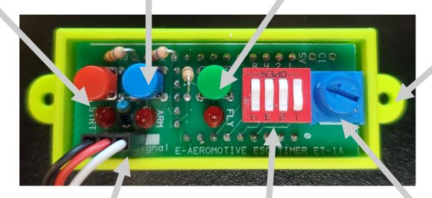
Mounting lugs (2) to secure unit to aircraft
